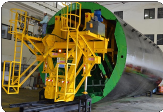
Tunnel Lining Gantry
